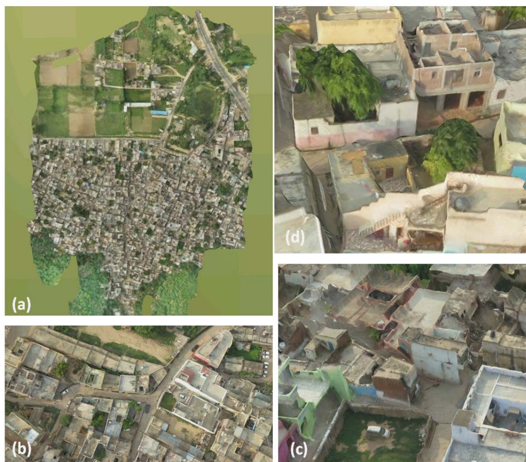
Fig 10 : (a) 3D Building of Bhondsi Village area processed using UAV images through Skyline City Builder and Photomesh software for Property and Land Management Applications (b) Zoomed Top View of the 3D Model of Bhondsi (c) & (d) Isometric View of few buildings in Bhondsi.
